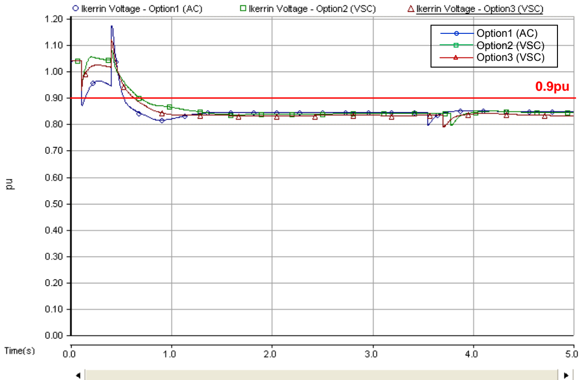
Figure 10.6: Ikerrin 110 kV bus voltage during the breaker failure at Cahir 110 kV terminal (Contingency 3_1_X in Table 10.1).
