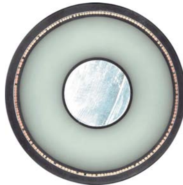
Figure 4-7 cross section of a 400 kV XLPE cable with 1200 mm 2 Al conductor (A2XS(FL)2Y, 3*1*1200 RE/50; source NKT Kabel)
