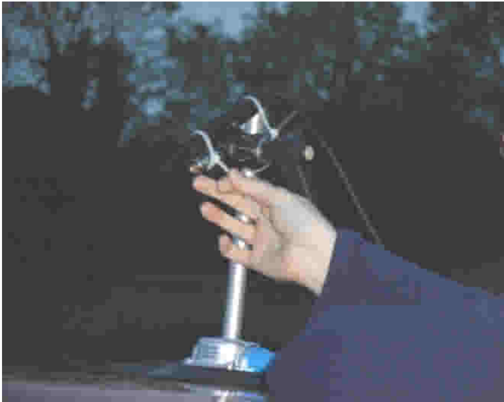
Photograph 1 – shows the external microphone for the Petterson D500x full-spectrum bat detector being secured to the attachment of the suction mounted support on the roof of a vehicle immediately prior to the commencement of a transect survey.
