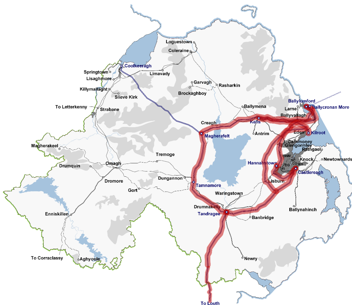
Figure 8.3: 275 kV circuits with works planned for RP7
