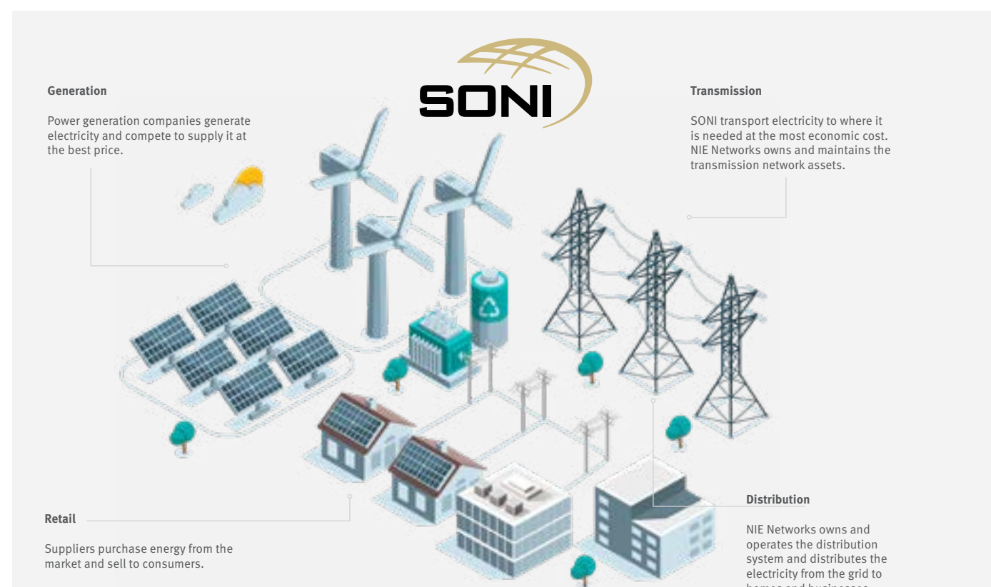
Figure 1: The structure of the electricity system in Northern Ireland
