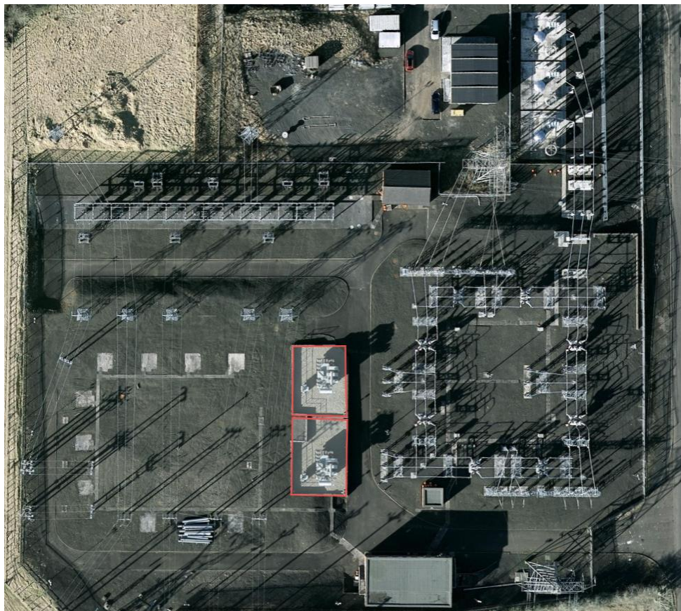
Figure 1 - Overhead image of Coleraine Substation. Transformers outlined in red
