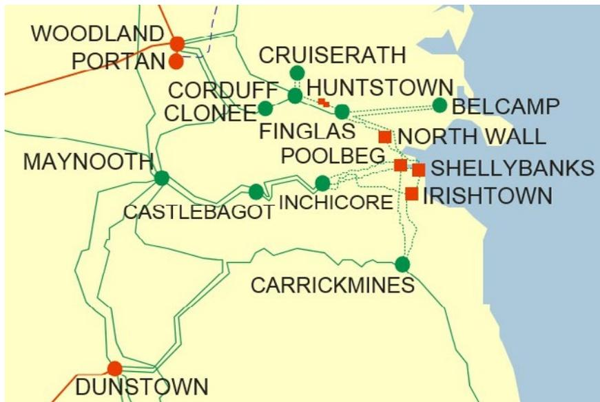
**Figure 8-2: Dublin Area 220 kV Transmission System**
