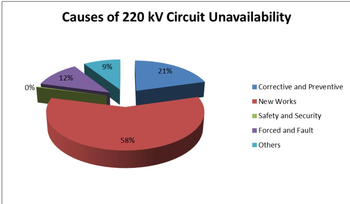
Figure 10: Causes of Unavailability on the 220 kV System in 2021
