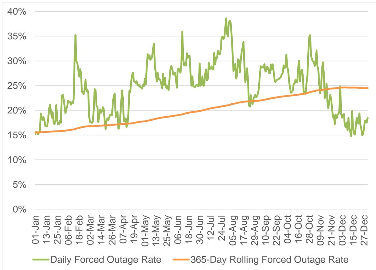
Figure 2: All-Island Dispatchable Generator and DSU Forced Outage Rate 2021
