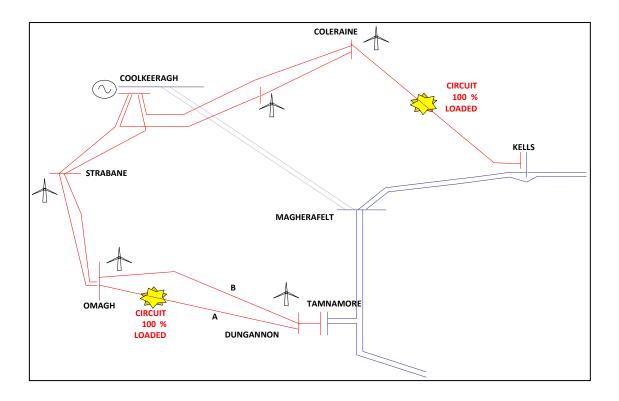
Figure 7: NW Network Map Showing Cause of Constraints
