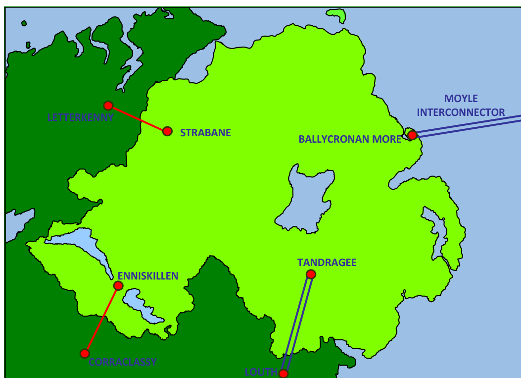
Figure 3.1: Existing Cross Border Circuits and Interconnection
