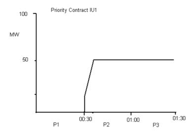
Note the ramp from 0MW to 15MW is instantaneous.
