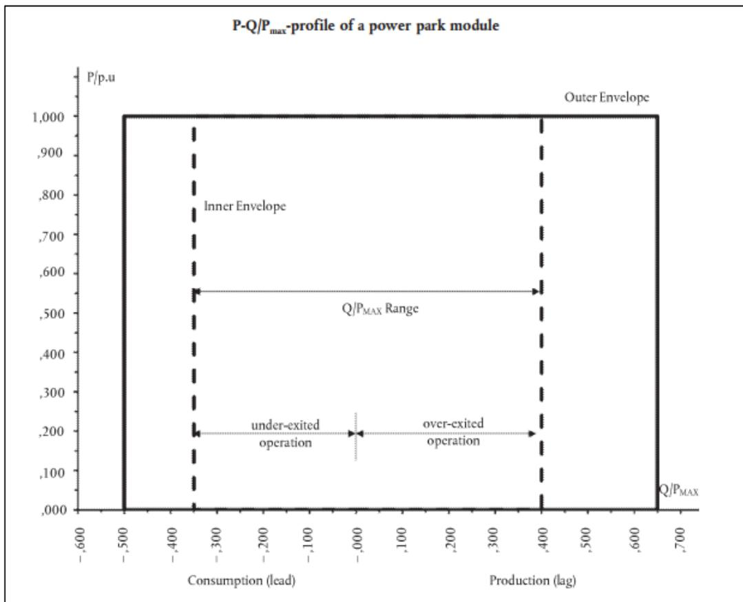
The diagram represents boundaries of a P-Q/P<sub>max</sub>-profile at the connection point by the fixed outer envelope.
