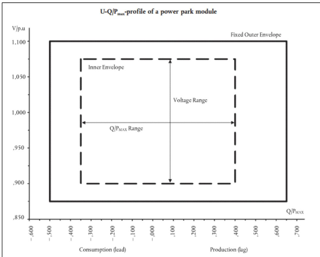
Figure 3: U-Q/P<sub>max</sub>-profile for Power Park Modules
