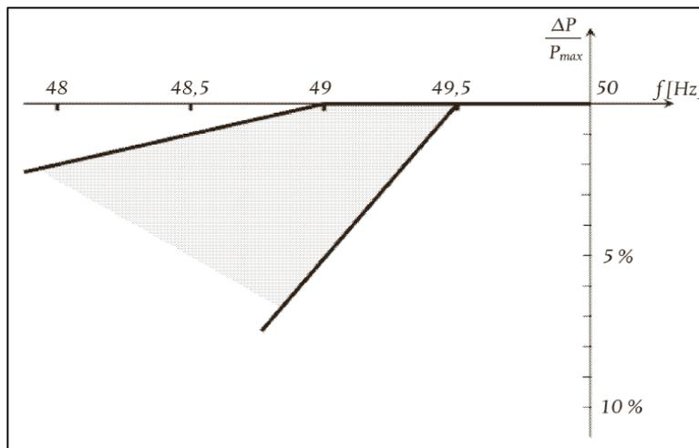
Figure 1 Maximum Power Capability Reduction with Falling Frequency
