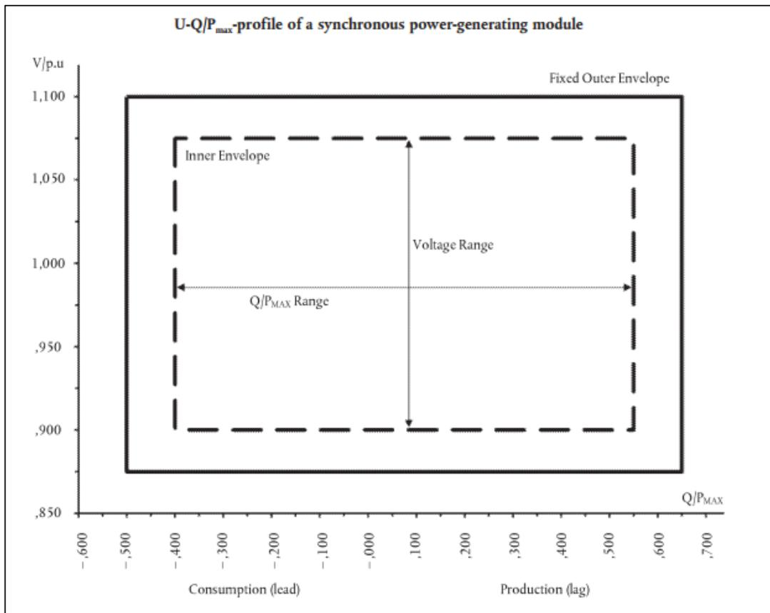
Figure 2: U-Q/P<sub>max</sub>-profile for synchronous Power-Generating Modules
