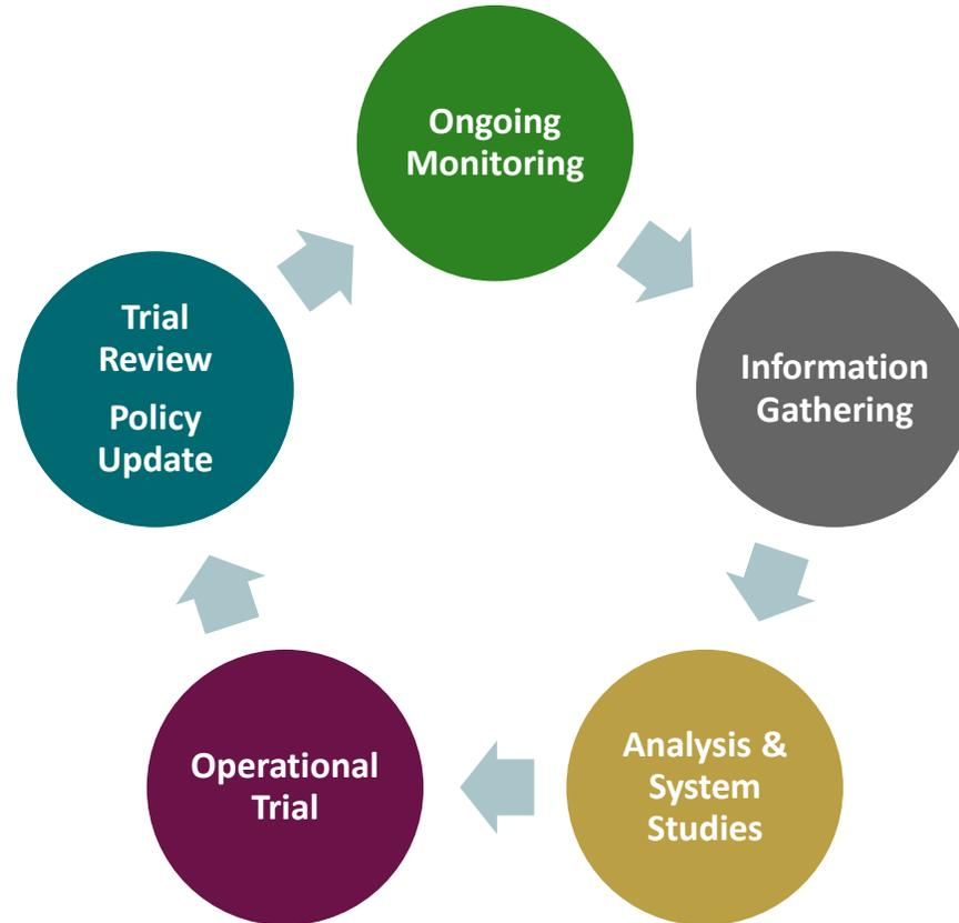
In the Ongoing Monitoring phase, EirGrid and SONI monitor the system parameters and analyse events and disturbances to assess system performance and generator compliance relative to operational policy parameters and metrics.
