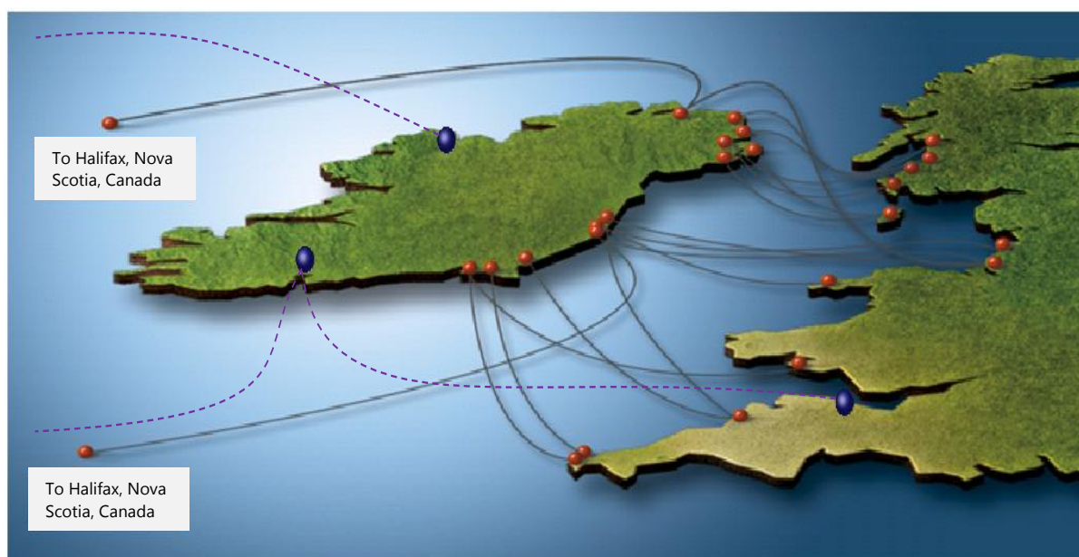
Figure 5-1 Ireland's offshore fibre connections as at Jan 2012 are illustrated with red boules, while the dashed lines depict the proposed Emerald Express & Project Express cables which may be on-stream by 2014.
