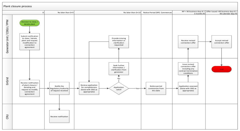
Figure 1 Generation Plant Closure Process Flow Chart
