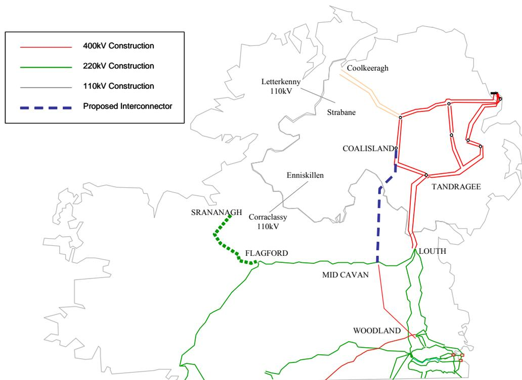
Figure 1: Network Schematic showing Proposed Interconnector
