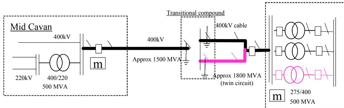
Figure A.4: Final Phase 400kV single circuit – increase to 1500 MW
