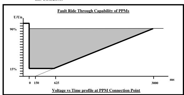
(b) **WFPSs** first connected to the **Transmission System** prior to 1 April 2005 shall not be required to comply with the requirements in the above diagram save where the **PPM** is subject to material modification involving the installation of
