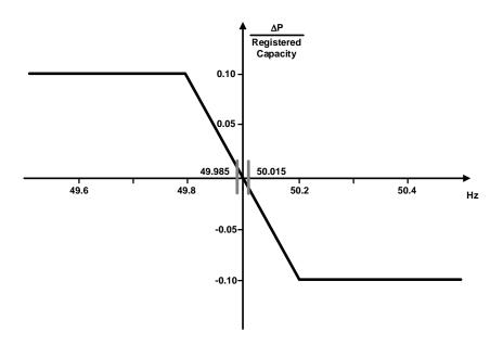
**Frequency** control devices (or speed governors) must be capable of operating to the parameters for **Active Power Frequency** response in **Frequency Sensitive Mode** as shown in the table below.
