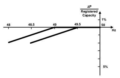
(c) For the avoidance of doubt, in the case of a **PPM** where the mechanical power input will not be constant over time, the requirement is that the **Active Power** output shall be independent of **System Frequency** under (a) above and should not drop with **System Frequency** by greater than the amount specified in (b) above.
